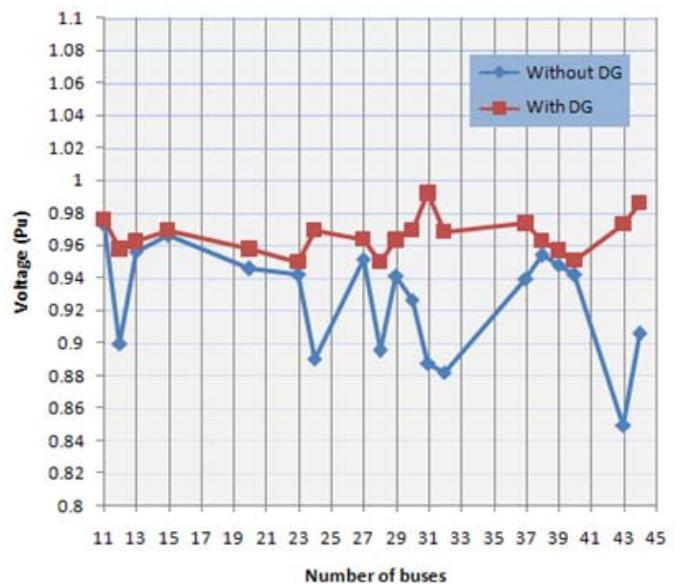
Figure 3- Voltage profile, before and after installing three DG resources
