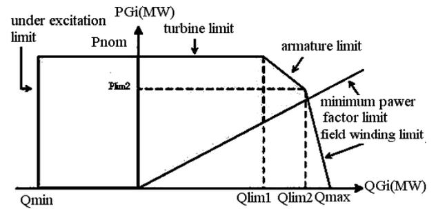
Figure 1- Constraint of exploiting a DG with a capacity of 1 MVA
