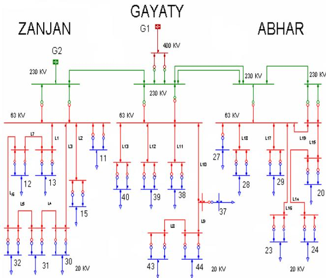
Figure 2- Single-line diagram of Zanjan Province network
