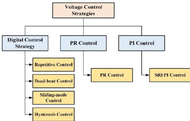
Fig. 6. Existing voltage control strategies for the outer voltage loop.
