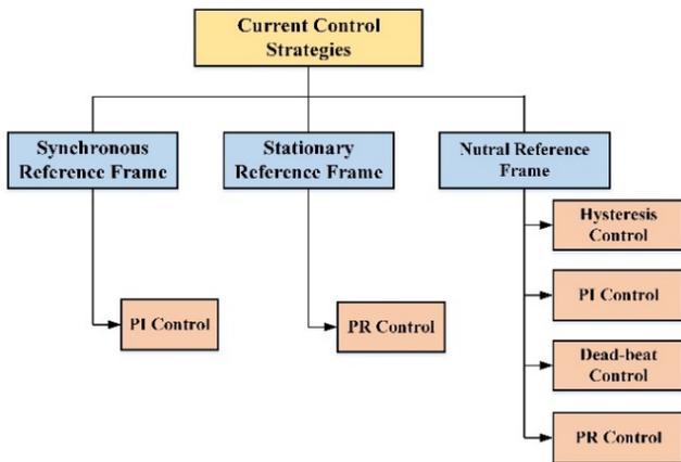
Fig. 5. Existing control strategies for the inner current loop.
