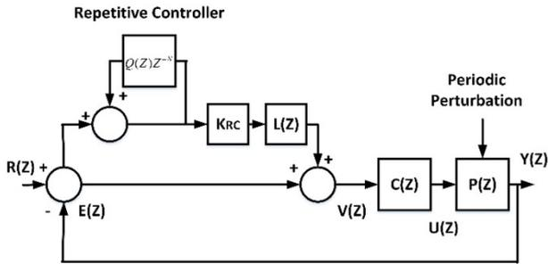
Fig. 7. Control diagram of repetitive control presented in [50].
