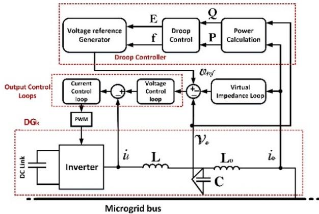
Fig. 2. Primary control: droop control with virtual impedance, and inner control loops applied to an inverter.
