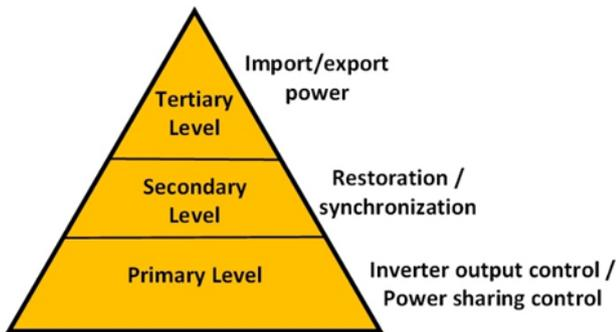
Fig. 1. Hierarchical control levels of a microgrid.
