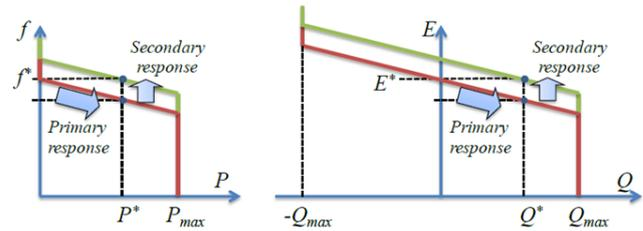
Fig. 3. P-f and Q-E primary and secondary control actions.
