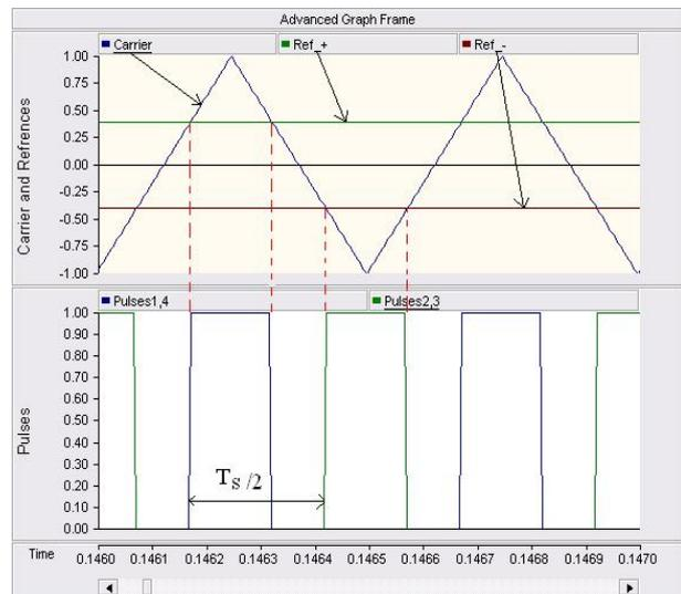
Fig. 3: PWM generation for full bridge converter
