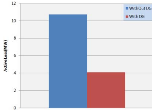
Fig. 7: The total active loss of the network, after and before installing DG resources.
