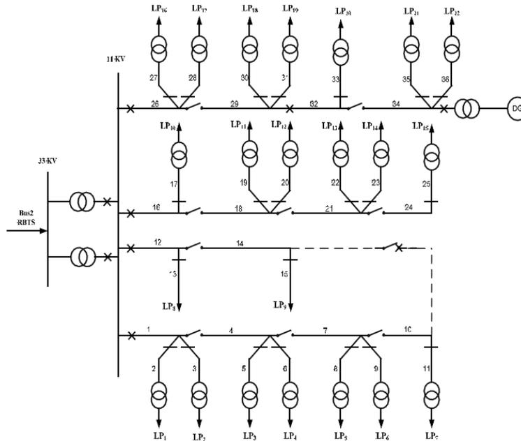
Fig. 2. Bus 2 of the standard distribution network of RTBS
